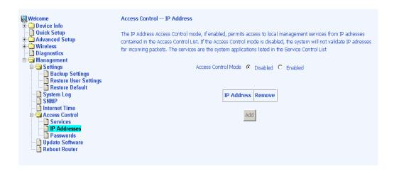
To assign the IP address of the management station that is permitted to access the local management services, enter the IP address in the box and click on the **Save / Apply** button.
